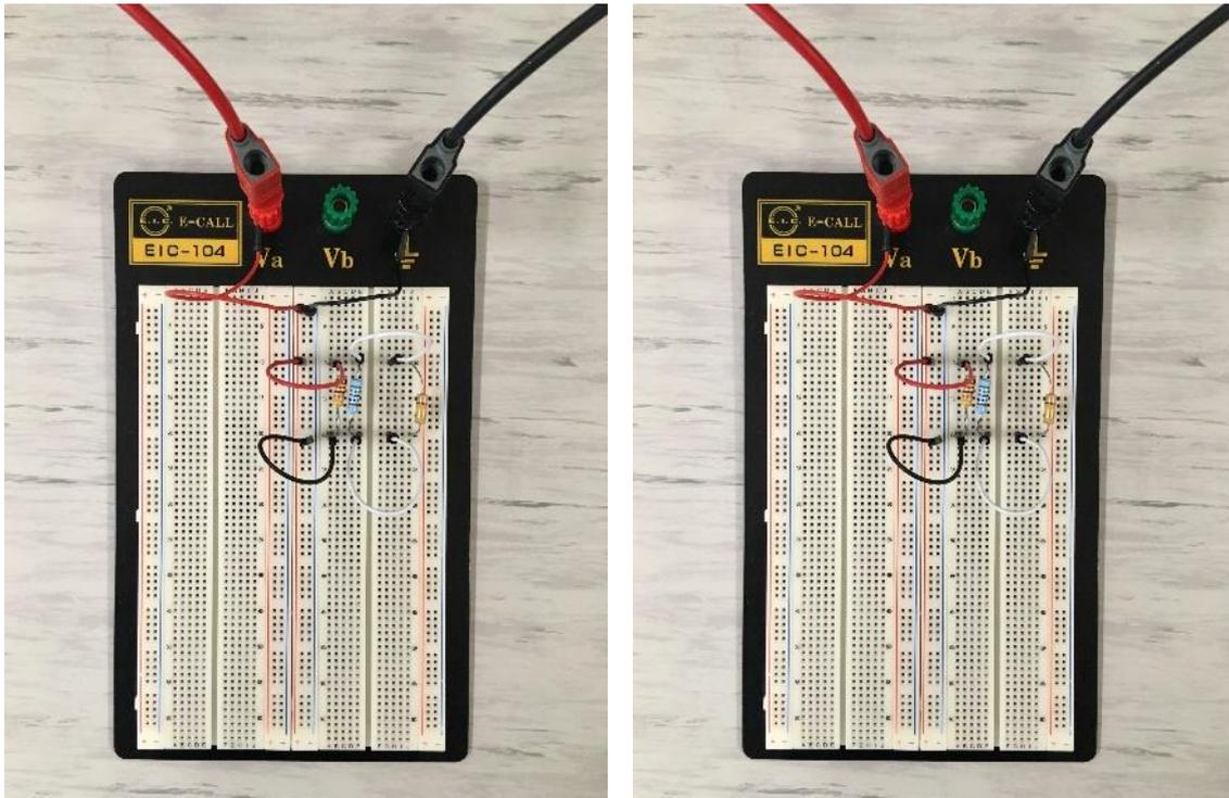
Figure 4.5: The parallel electrical circuit on protoboard
