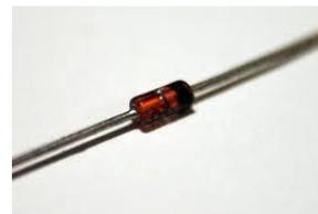
Figure 1.2: Appearance of diode
