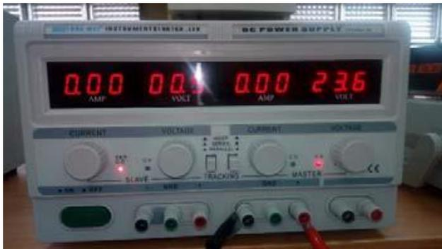
Figure 5.1 Variable DC power supply
