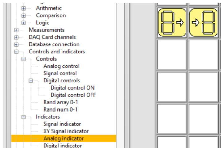
Figure 5.6 Desktop after setting < Analog indicator > indicator
