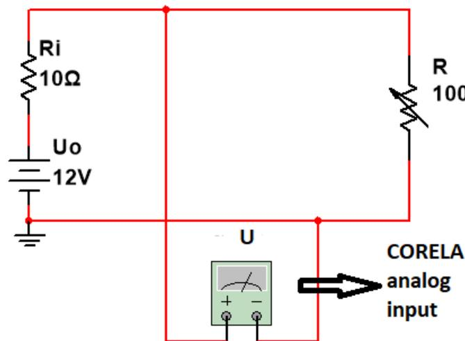
Figure 4.1: Wiring diagram for performing practical measurements
