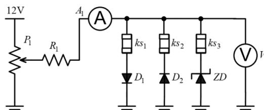
Figure 3.1: Electrical circuit for measuring static diode characteristics
