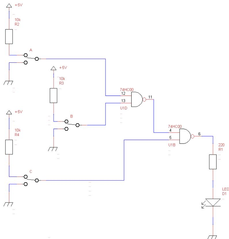
Figure 3.1.5: Schematic diagram of the logic function in purely NAND form and the electronic circuit
