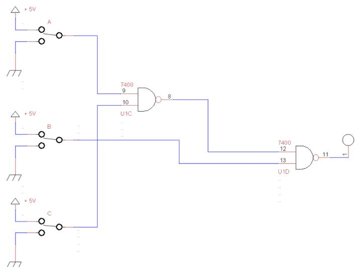
Figure 1.4.1: Schematic diagram of the logic function in the full disjunctive normal form implemented in purely NAND gate form and the electronic circuit
