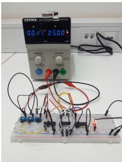
Figure 3.1.3: DC voltage power supply and the electric circuit on protoboard
