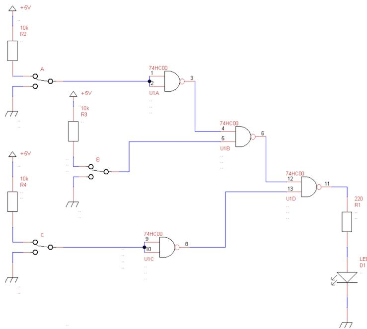
Figure 3.2.1: Schematic diagram of the logic function in purely NAND form and the electronic circuit
