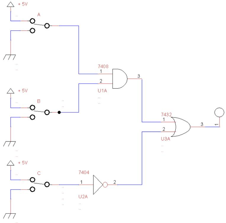
Figure 1.1.1: Schematic diagram of the logic function and the electronic circuit
