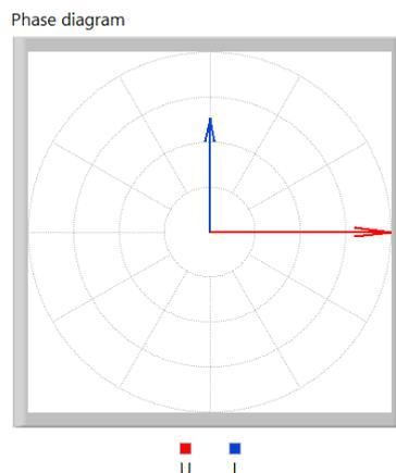
Figure 4.3: Phase diagram of an electrical circuit with a capacitor
