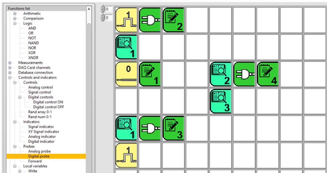
Figure 2.3.3: Notation of the logic function in the CORELA simulation editor
