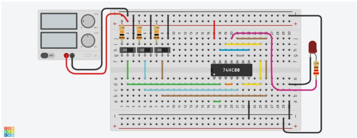
Figure 3.2.2: Scheme of the electric circuit on protoboard.
