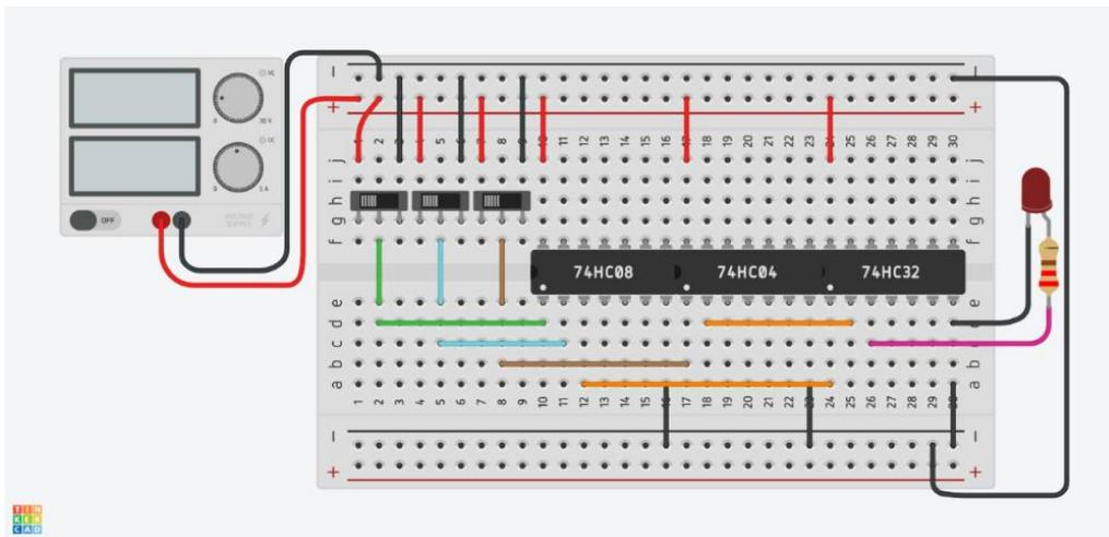
Figure 1.1.2: Scheme of the electric circuit in Tinkercad circuit simulator
