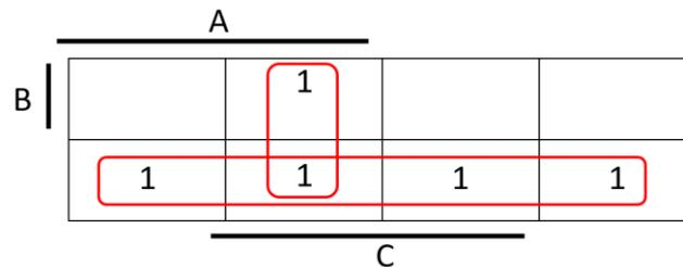
1.4.3) Write down the full disjunctive normal form. Simplify the logic function using Boolean algebra laws.
