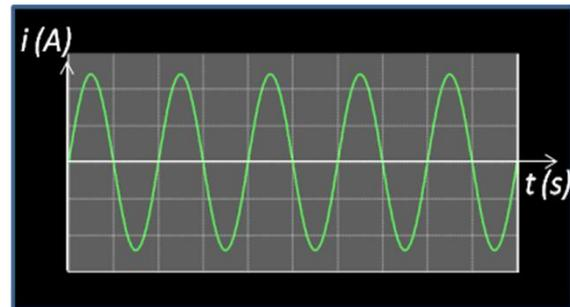
Figure 1.1: Sine wave alternating current
