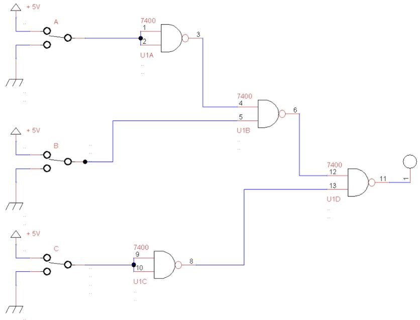
Figure 2.2.1: Schematic diagram of the logic function in purely NAND form and the electronic circuit
