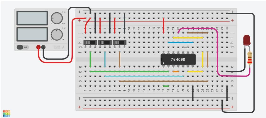
Figure 1.2.2: Scheme of the electric circuit in Tinkercad circuit simulator
