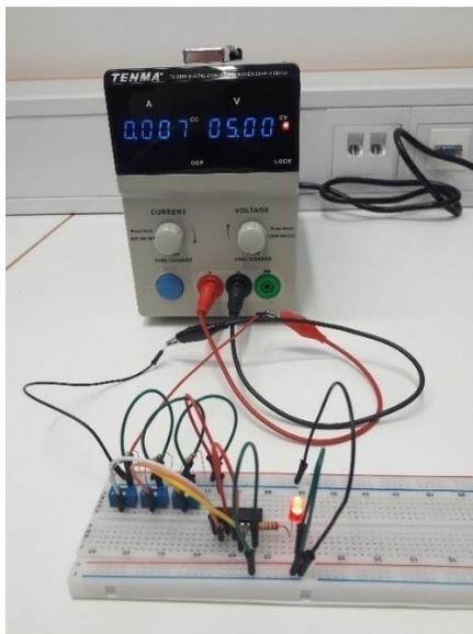
Figure 3.1.7: DC voltage power supply and the electric circuit on protoboard
