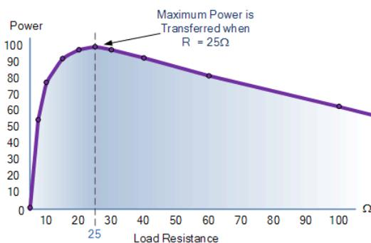
Figure 1.2: Graph of power against load resistance
