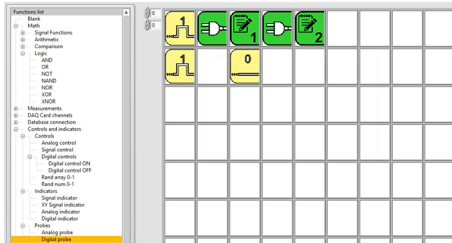
Figure 2.1.4: Notation of the logic function in the CORELA simulation editor
