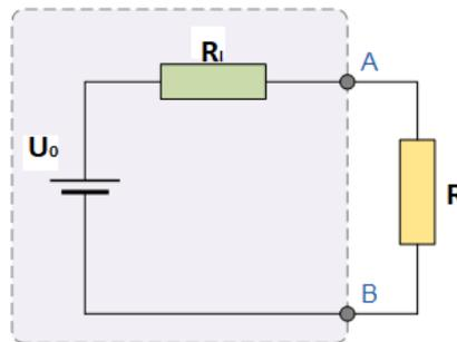
Figure 1.1: Replacement scheme of real source with load
