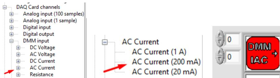
Figure 5.4: Activation of digital amperemeter with a measuring range of 200mA
