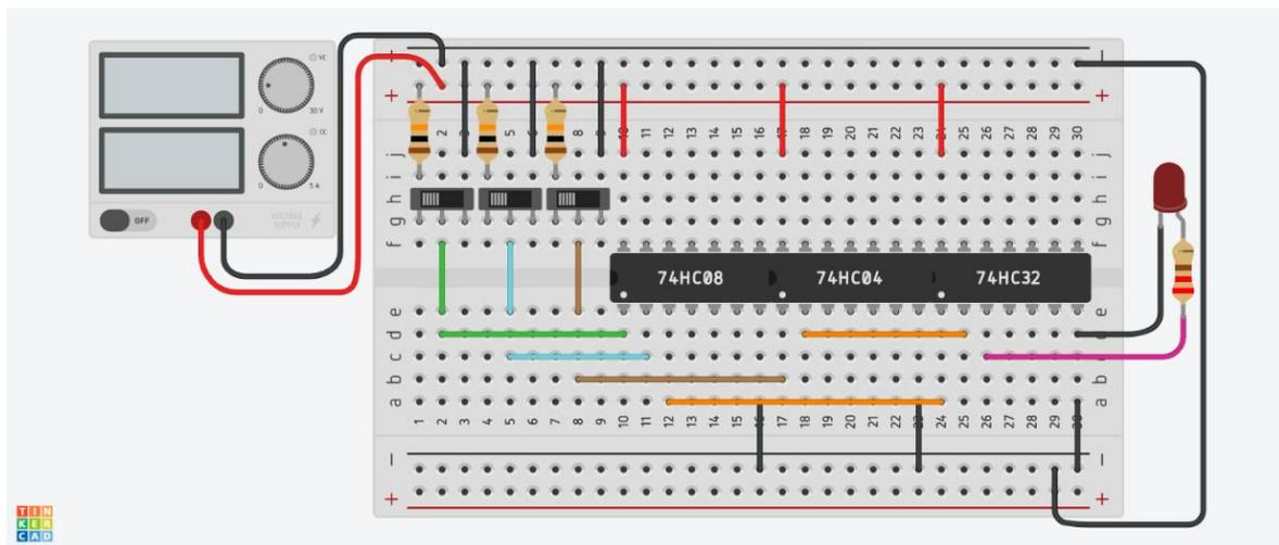
Figure 3.1.2: Scheme of the electric circuit on protoboard
