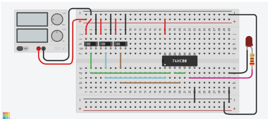
Figure 1.1.4: Scheme of the electric circuit in Tinkercad circuit simulator
