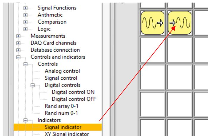
Figure 3.5: Access to entered data with Signal indicator function
