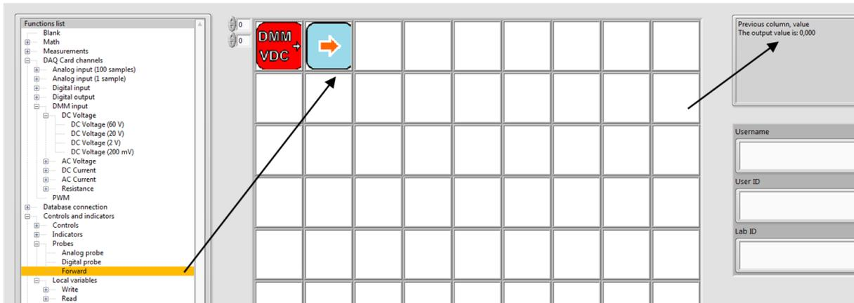
Figure 5.8: Reading the measured voltage value from message box
