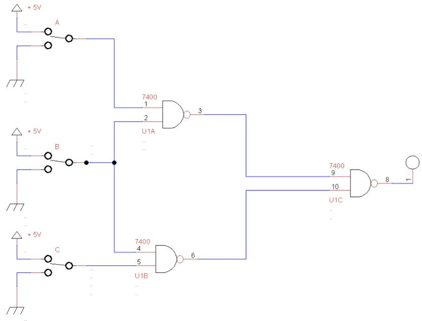
Figure 2.3.2: Schematic diagram of the simplified logic function in purely NAND form and the electronic circuit
