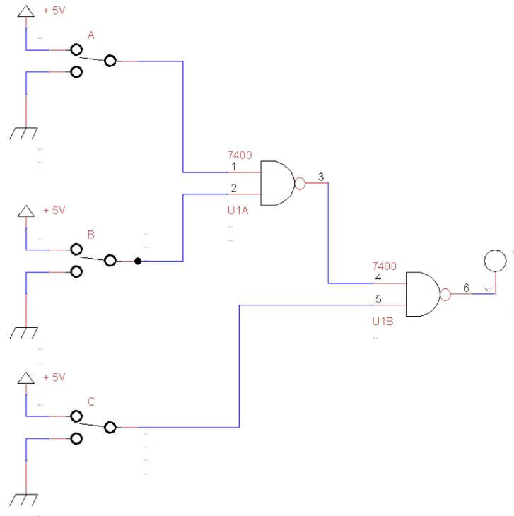
Figure 1.1.3: Schematic diagram of the logic function in purely NAND form and the electronic circuit
