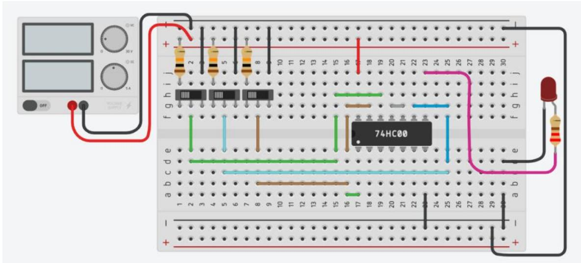
Figure 3.4.2: Scheme of the electric circuit on protoboard
