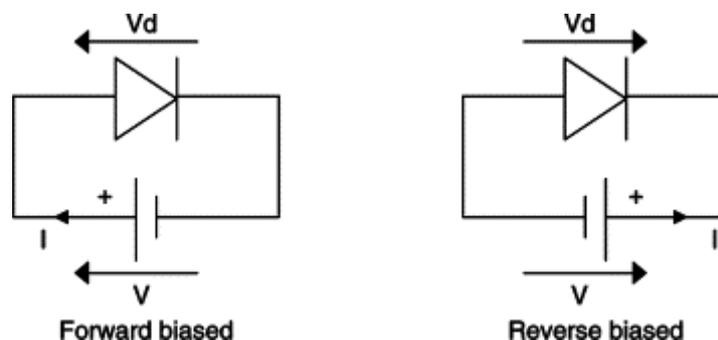
Figure 1.3: Direct and inverse polarized diode
