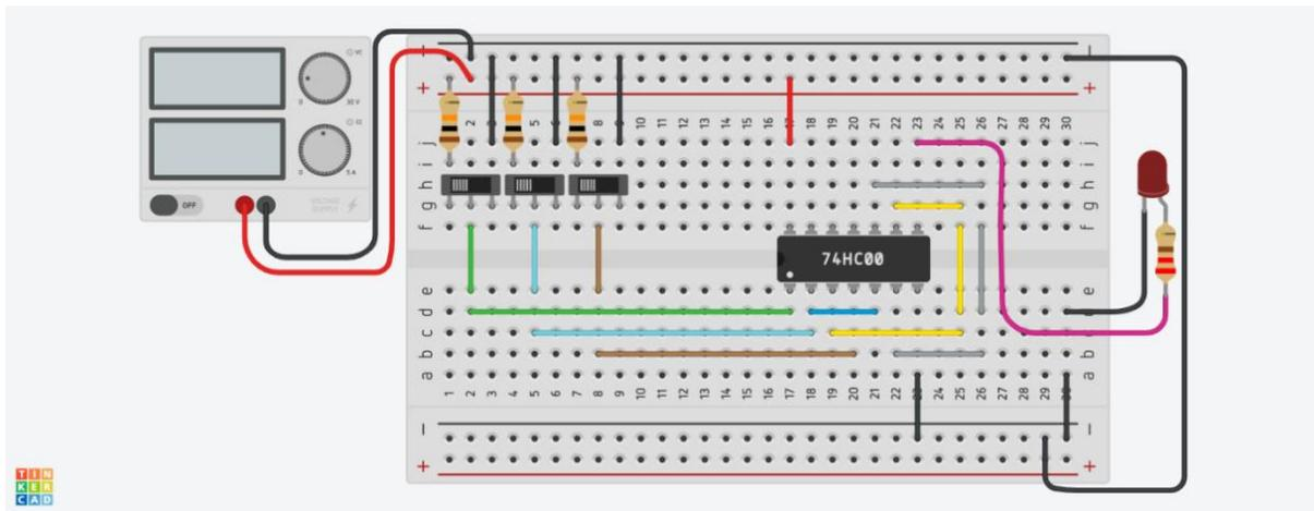
Figure 3.3.3: Scheme of the electric circuit on protoboard
