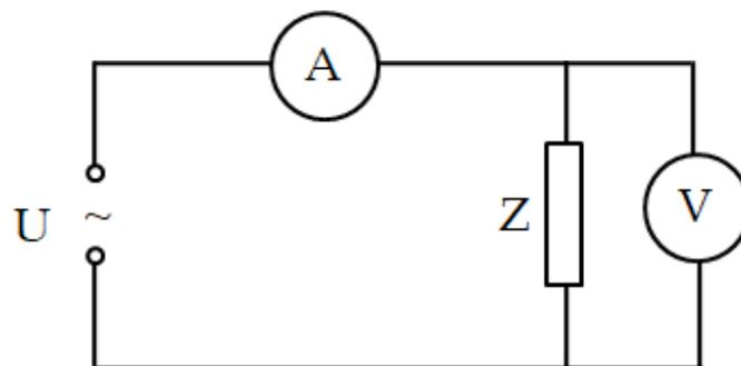
Figure 5.1: Electrical circuit for impedance measurement
