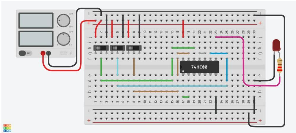
Figure 1.4.2: Scheme of the electric circuit in Tinkercad circuit simulator.
