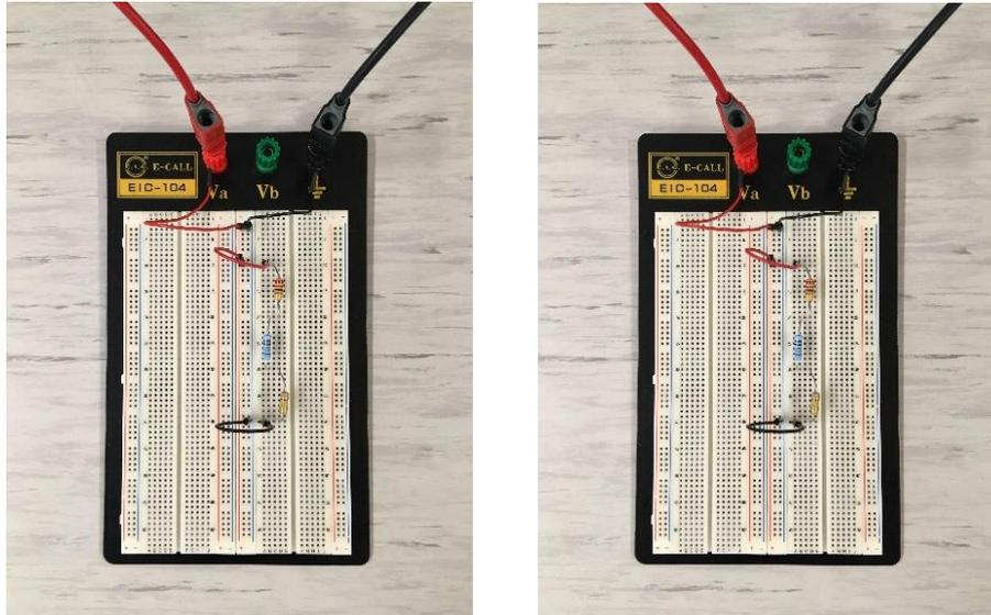
Figure 4.3: The series electrical circuit on protoboard
