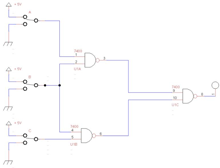
Figure 1.3.2: Schematic diagram of the simplified logic function in purely NAND form and the electronic circuit
