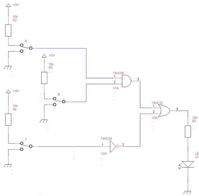
Figure 3.1.1: Schematic diagram of the logic function and the electronic circuit
