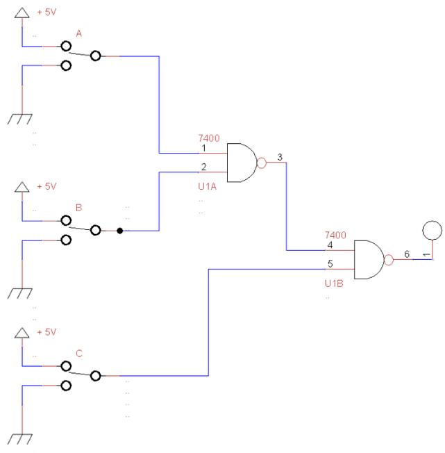
Figure 2.1.3: Schematic diagram of the logic function in purely NAND form and the electronic circuit
