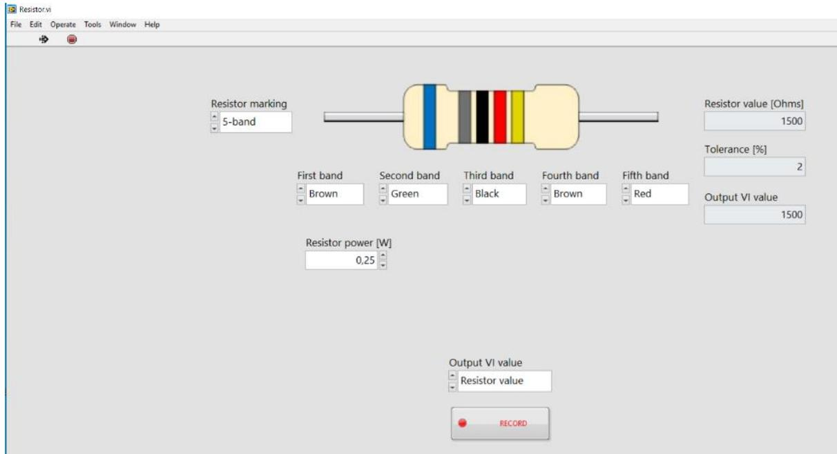
Figure 3.1: Resistor value determination
