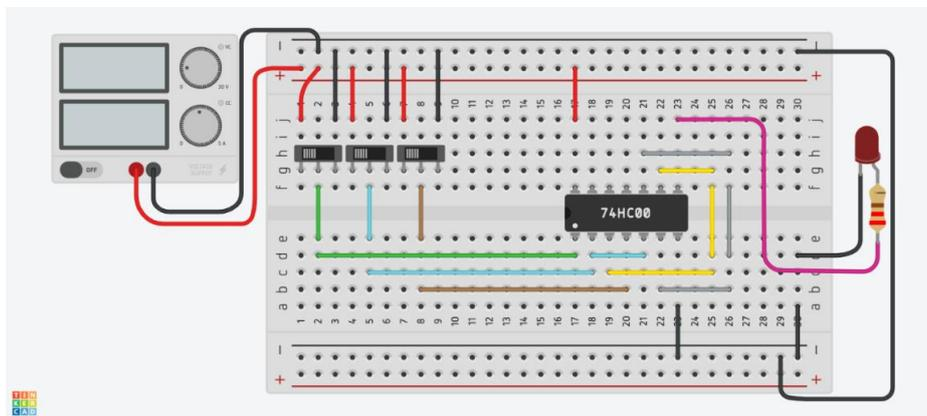
Figure 1.3.3: Scheme of the electric circuit in Tinkercad circuit simulator
