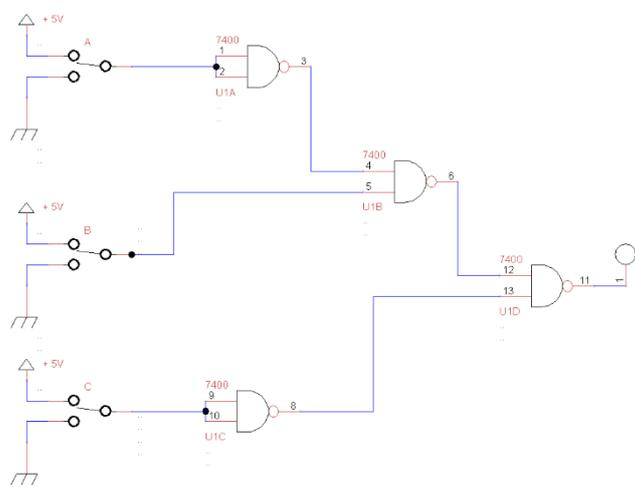
Figure 1.2.1: Schematic diagram of the logic function in purely NAND form and the electronic circuit
