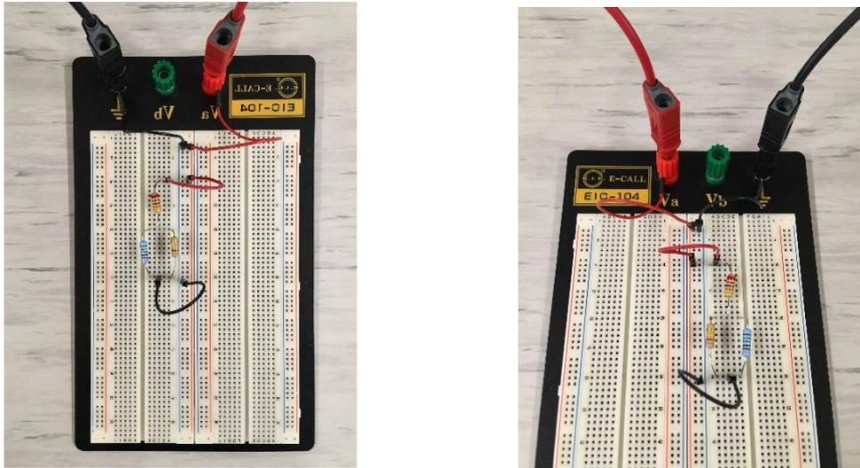
Figure 4.7: The series-parallel electrical circuit on protoboard
