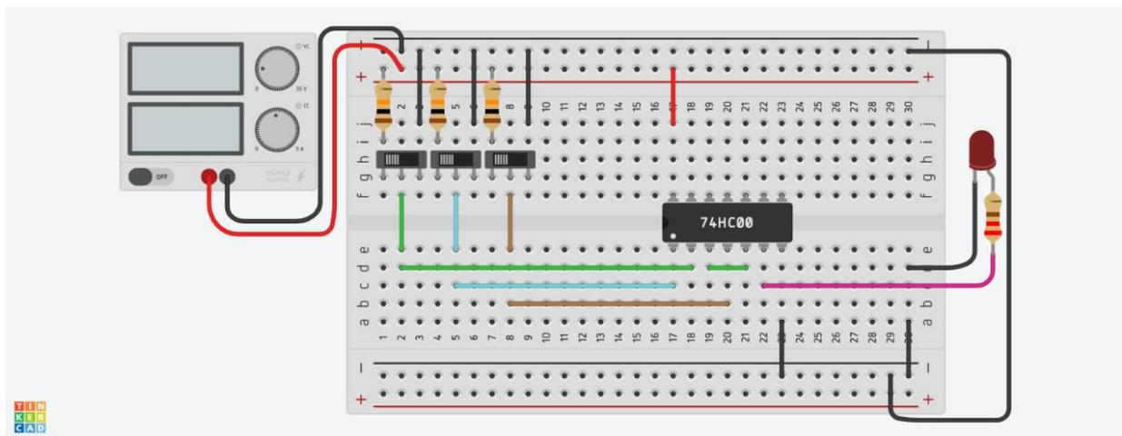
Figure 3.1.6: Scheme of the electric circuit on protoboard
