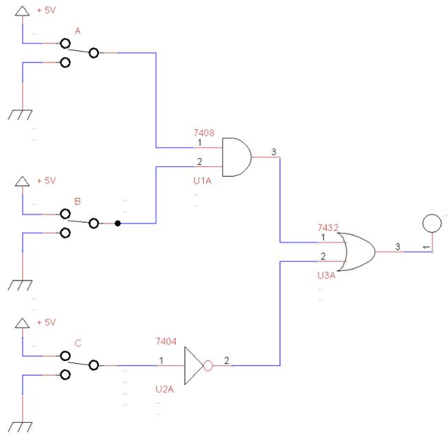
Figure 2.1.1: Schematic diagram of the logic function and the electronic circuit
