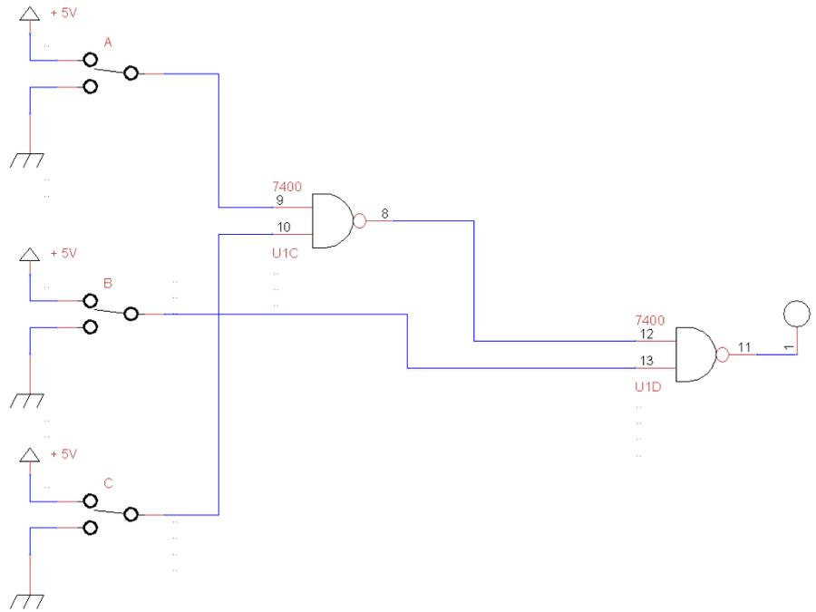
Figure 2.4.1: Schematic diagram of the logic function in disjunctive normal form implemented in purely NAND gate form and the electronic circuit
