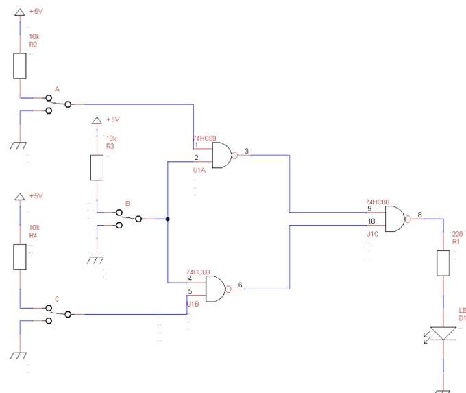
Figure 3.3.2: Schematic diagram of the simplified logic function in purely NAND form and the electronic circuit
