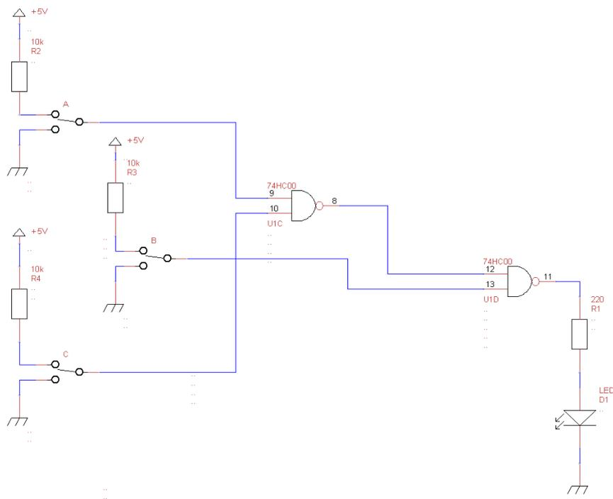
Figure 3.4.1: Schematic diagram of the logic function in the full disjunctive normal form implemented in purely NAND gate form and the electronic circuit
