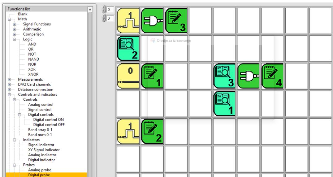
Figure 2.4.2: Notation of the logic function in the CORELA simulation editor
