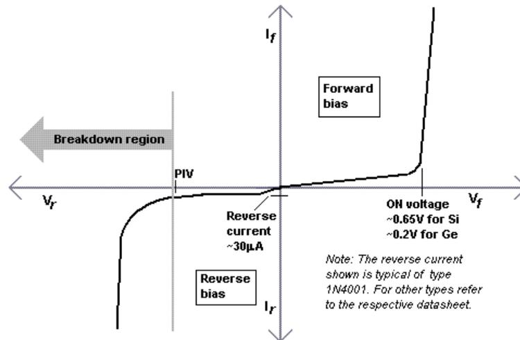
Figure 1.4: Static current - voltage characteristic of the 1N4001 diode
